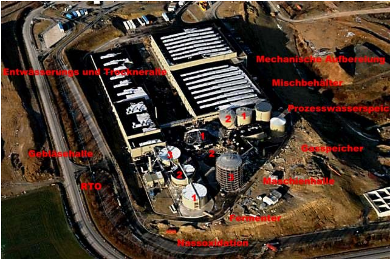
Figure 3. Aerial photo of the MBP-/ MBT-plant after the accident, showing the drawn layouts of the parts of the plant
